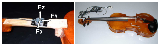
Figure 1. The violin with a 3-D force transducer
